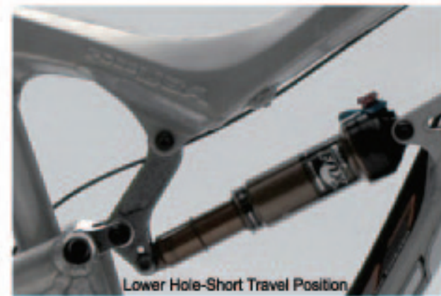
Lower Hole-Short Travel Position 5"/ 127mmTravel
