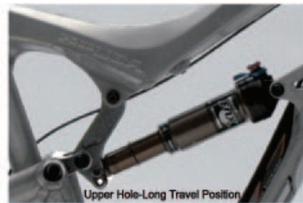
Upper Hole-Long Travel Position 5.5"/ 140mmTravel
