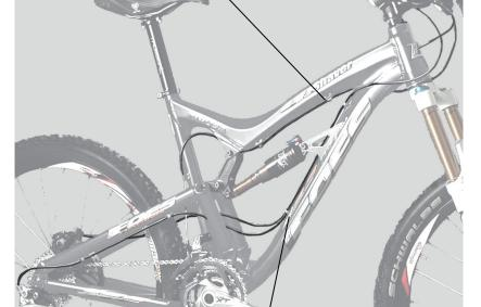
Down Tube Cable Guides 1: for Rear Derailleur Cable 2: for Rear Disc Brake line
