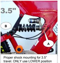
travel. ONLY use LOWER position in main frame (A) and LOWER position in swingarm (B) as pictured. Make sure shock reservoir is facing up as shown.
