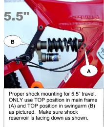
Note: Changing travel positions may require changing spring rates and compression/rebound damping settings. This may mean purchasing a different spring than we ship with the frame.
